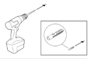
3 Use a Phillips-head screwdriver or power drill to screw in the wall mount bracket.
