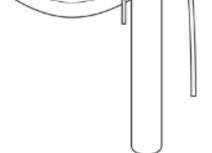
Press the power cord into the stem, working from top to bottom. Pull the excess cable down from the base.
