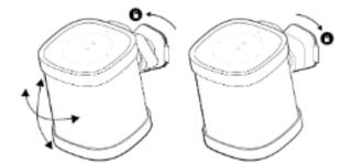
8 Route the power cable into the side hook and plug the speaker into power.
