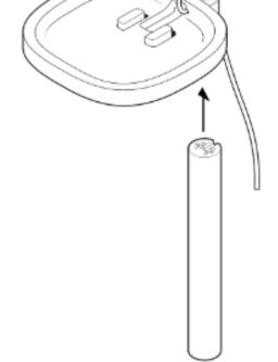
Use the 2 silver screws to attach the speaker platform to the top of the stem, threading the power cable carefully. Snap the bottom plate on with the power cable channel in the back, and mount the platform on the stem.
