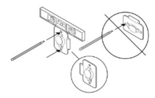
If you're using wall anchors, use a 5/16" drill bit to drill 2 pilot holes and then insert the wall anchors.
