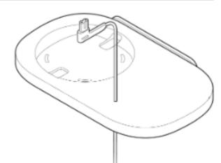
Carefully align the pins, then press the bottom cover firmly onto the shelf until it snaps into place. Plug the power cord into the speaker and place it on top of the Shelf.
