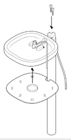
Plug the power cord back into the speaker and place on the top mount, pulling any extra cable down from the top. Tighten the screws and attach the top cap with the notch facing toward the speaker.
