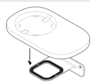
Route the speaker's power cord through the Shelf opening. (You'll wrap the cord around the bottom of the Shelf after it's assembled.)
