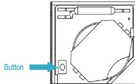
Identify the device by pressing the button 4 times while its identify window is open. The device's 64-bit address should appear in the identify window's text box.
