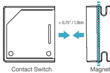
Install the magnet in the proper orientation using 2-sided tape or screws. The magnet must be within 0.75" (1.9 cm) of the Sensor.
