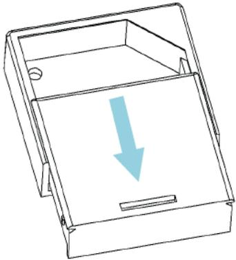
Slide open the Door/Window Sensor's top housing. Install the CR2032 battery in the housing top as shown below.
