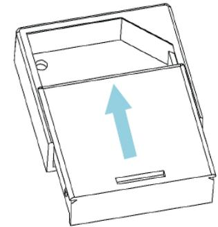
Once you have confirmed the device is communicating, insert the sensor top housing as shown above
