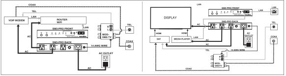
Sample setups to indicate the basic configuration for proper connections. Protecting all AC and signal lines will keep your system safe and ensure compliance with Panamax's Connected Equipment Policy.
