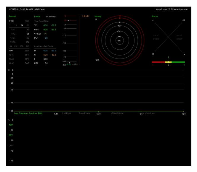
The only detectable readings we see above are the self-noise of the test equipment itself. It's essentially zero.
