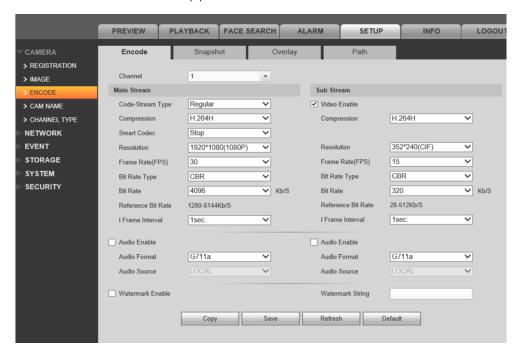
*Video Stream Settings:* Configuration of the video streams is recommended. Below are the typical settings an installer should set the video to:
