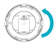
Remove the Mounting Plate by rotating the Housing counter-clockwise as shown.
