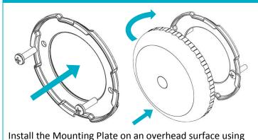
the two #6 screws provided. Place the Sensor Housing over the Mounting Plate, there is no "keyed" location. Rotate the Housing clockwise to lock it into place.
